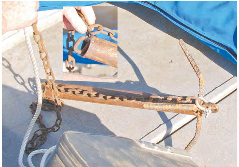
Grapple anchors work best when the claws dig into the bottom structure, but they can also get hung and can be lost.
