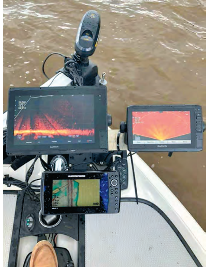
The bow of Tim Hebert’s boat looks more like an airplane with the LiveScope down chart (upper left), perspective mode (upper right) and Humminbird Helix Sonar (bottom).
